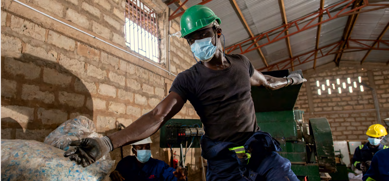
An ASASE worker feeds plastic flakes into an extruder.
