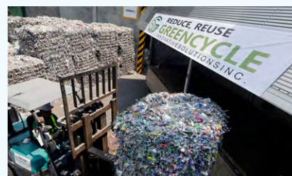
Bales of plastic scrap, soon to be turned into RDF for cement kilns.
