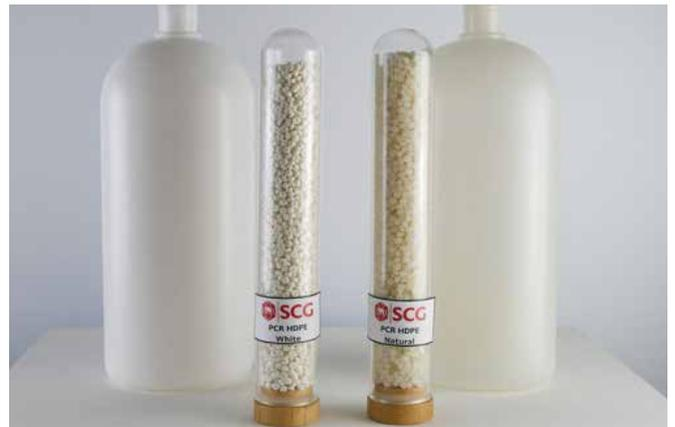
SCGC has developed advanced recycling/chemical recycling for difficult-to-recycle plastics like multi-material packaging, which can turn used plastic into recycled feedstock through a petrochemical plant process into plastic resin with the same properties as virgin ones. This recycled plastic resin's manufacturing process and properties are certified by ISCC PLUS, the International Sustainability and Carbon Certification (ISCC), making it the first in Thailand to fulfill these criteria.
