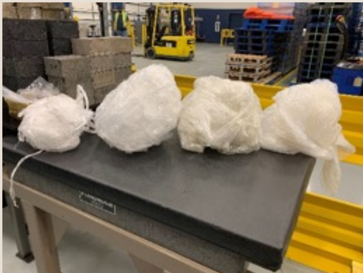
Figure 3: Machine-applied shrink film uses half of the material than a hand-applied alternative (from left to right: Control machine-applied, control hand-applied, PCR, compostable)
